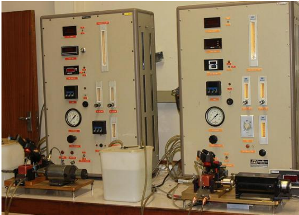
Figure 1: Image of the BOCLE (left) and SL-BOCLE (right) (Langenhoven, 2012).
