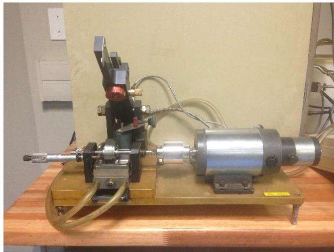
Figure 2: Ball-On-Cylinder configuration (Actual photograph taken at the Tribology lab)
